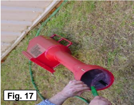
Figure 15 - Clean the back of the hopper with a watering hose
