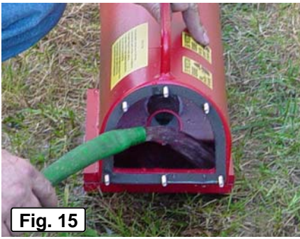
Figure 15 - Clean the back of the hopper with a watering hose
