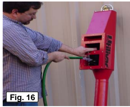
Figure 16 - Cleaning the under-side with a watering hose. Use soap and water.
